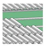
Right Start<sup>®</sup> UDL is mechanically fastened to the roof deck, and carries a **UL Class A Fire Rating** when installed with a fire-rated roof covering.
